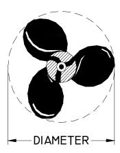
Pitch = 17 Diameter = 14 Pitch and Diameter are the two basic dimensions of a propeller. Example of propeller dimension:  $14 \times 17$
